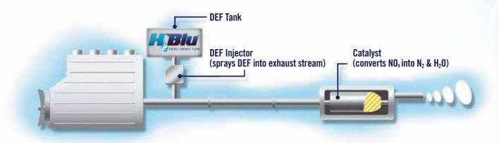
SCR technology reduces the concentration of nitrogen oxide ( $NO_x$ ) gases that are produced inside the engine during combustion. This process requires the right amount of DEF to be injected into the exhaust stream. Upon mixing with exhaust gases, it is hydrolyzed before the catalytic converter breaks down nitrogen oxide ( $NO_x$ ) into harmless nitrogen ( $N_2$ ) and water ( $N_2$ ).
